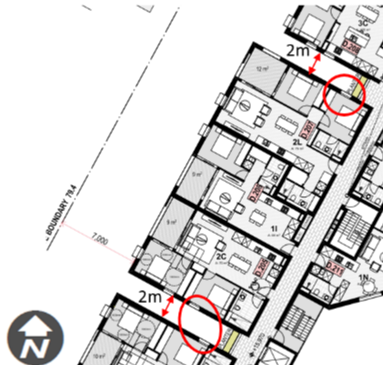
Figure 34: Original Level 2 plan with slots in the western portion of the proposed development
